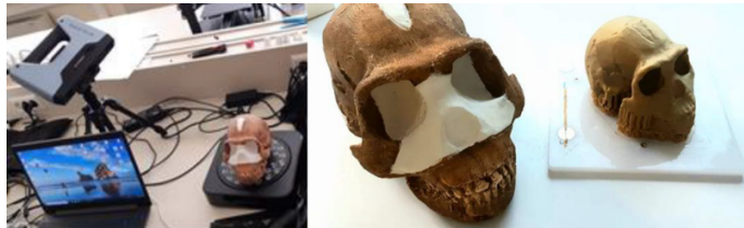
Fig. 2. Experimental setup used to measure the cranium in 3D and Homo naledi cranium (left) and 3D printed replica of skull as it was removed from the 3D printer (right)
